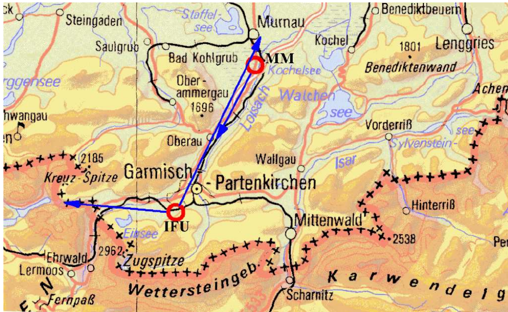
Figure 3.68: Map of the mountains around Garmisch-Partenkirchen and the Loisach valley; the positions of the two aerosol lidars are marked by circles, the three principal scanning directions by arrows. From the scans along the valleys a two-dimensional map of the backscatter coefficients will be generated.
